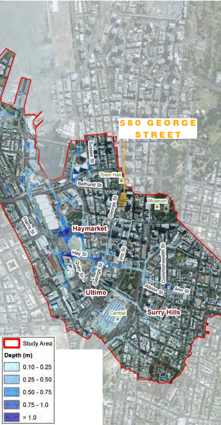
PEAK FLOOD DEPTH 1% AEP DESIGN FLOOD EVENT
